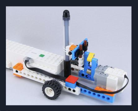
Adjust the position of the pen so that the tip doesn't touch the surface of the paper when the pen holder is up and does when they holder is down.
